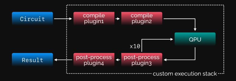
Extension of any QPU object to a stack my\_stack = plugin1 | plugin2 | plugin3 | plugin4 | my\_qpu
